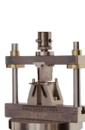
短梁层间剪切夹具 ASTMD2344, ISO14130, EN2563, EN2377
