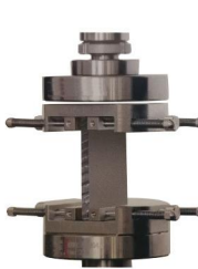
层板侧压夹具 ASTM C364
